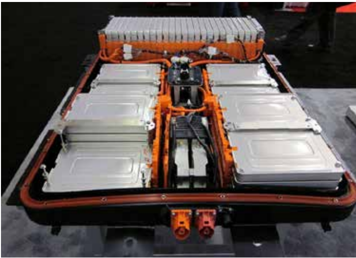
This is a photo of the Nissan Leaf's li-ion battery pack. The Leaf was introduced in 2011 as the first mass-produced EV sold in the U.S. In 2026, Nissan will begin building two new EV models at its plant in Canton, Mississippi.
